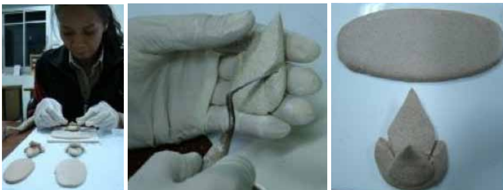
Figure 6. Specialists in Thai traditional stucco is testing Re-Material Paper Stucco.
