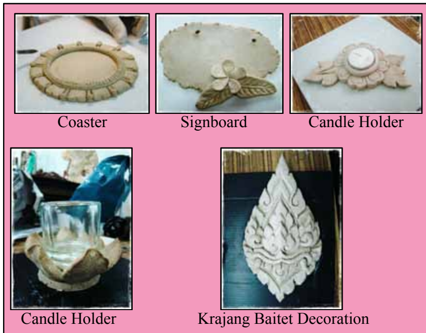
Figure 10. Sample products made from Re-Material Paper Soil that were accepted by the Stucco experts.
