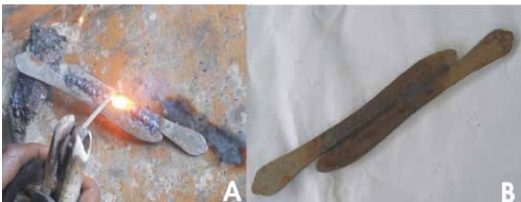
Figure 5. Arc-welding of stainless-steel knives (A), welded knives (B).
