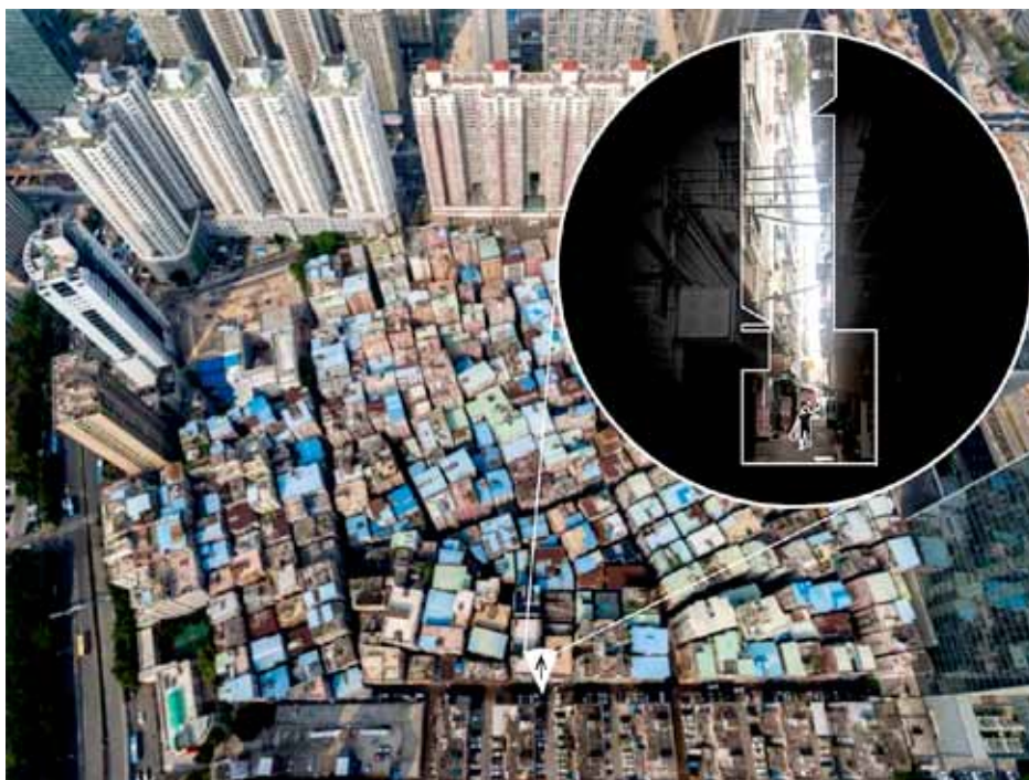
Figure 5. The low Sky View Factor (SVF) in Shenzhen Urban Village. Source: Illustration is created by Authors, the aerial view photo from “Urban Mountains,” (2018) photographer Li Zhenxing, and the eye view photo from Zhang (2019) photographer Phoebe Zhang.
