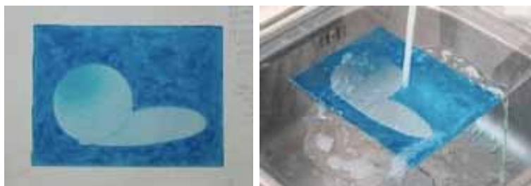
Figure 13. The plate coated with the mixture of Winson Screen Filler no.67 and water (left); the coating could be easily washed out by water (right).
