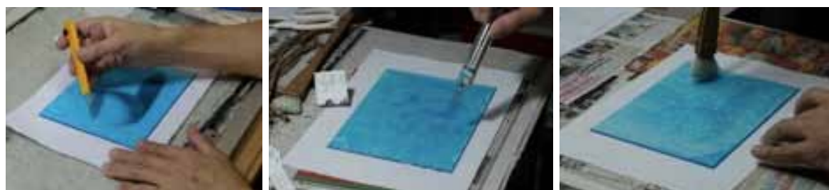
Figure 5. Scratching through the coating with a cutter (left); dichloromethane dripping (center); brushing off the residue (right).
