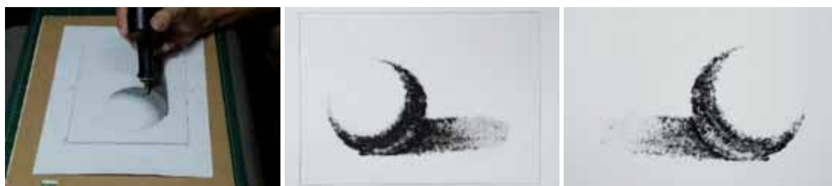
Figure 4. An electric carving & marking pen (left), the plate (center) and printing results (right).
