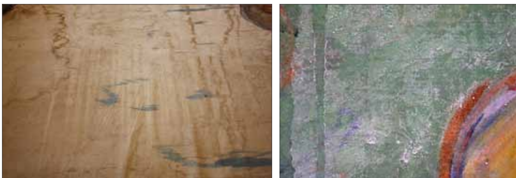
Figure 5. Left, Drain marks, water stains, deformations and folds. Photo: Eva Storevik Tveit and Figure 6. Right, White surface material/salt efflorescence. Photo: Erika Gohde Sandbakken.
