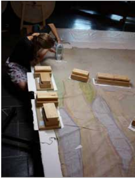
Figure 14. Flattening the folds with weights. In the background measurements with a hand-held x-ray fluorescence analyzer (XRF-instrument). Photo: Lina Flogstad.
