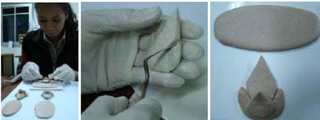
Figure 6. Specialists in Thai traditional stucco is testing Re-Material Paper Stucco.
